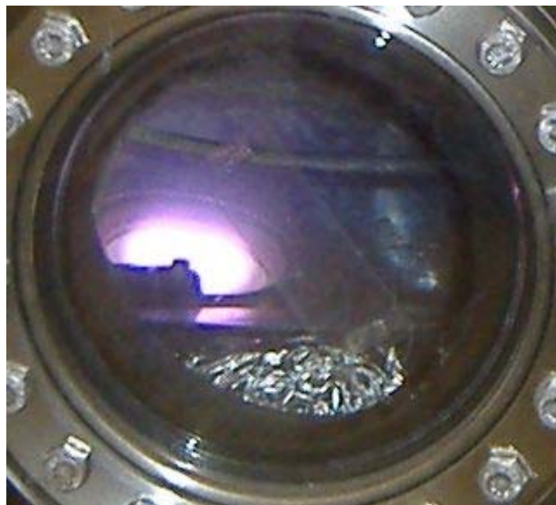
Figure 2.5 Plasma Formation in the Chamber
